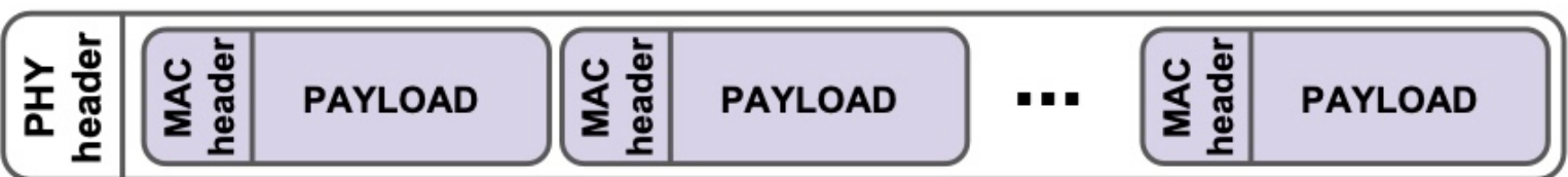
Figure 1: 802.11n/ac A-MPDU structure
